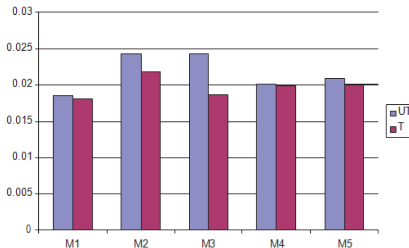
Figure 3. Dry thermal resistance of untreated and moisture management finished (MMF) fabrics (X-axis = different type of knitted fabrics, Y-axis = dry thermal resistance, m 2 K/W).
